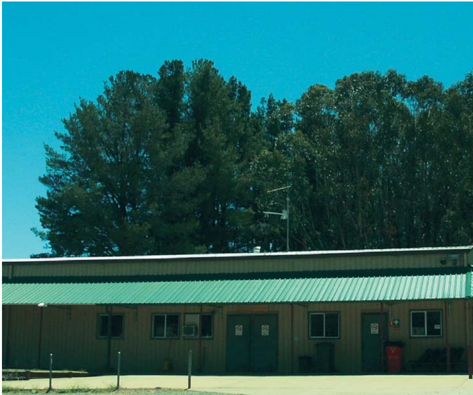
Figure 1. Location of Bondo weather station (WS) wind sensors on roof of building at the FNSW Bondo Ranger Station. Note row of dense canopy north of the sensor.
